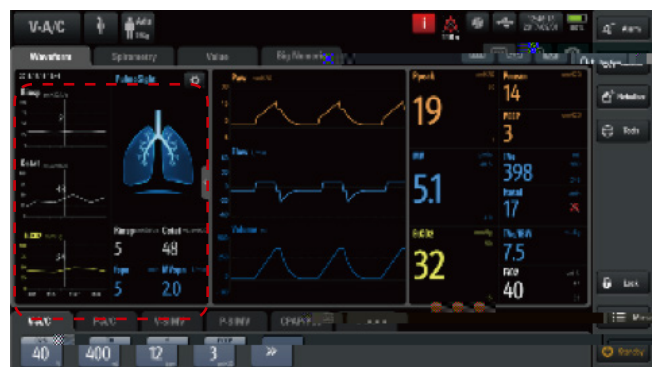
PulmoSight in the Mindray SV Series ventilators can closely monitor the changes of respiratory mechanics and display the data in a real-time, graphic way.
